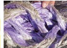
Inspection of hollow core area of Plasma® 12x12 rope. In picture above, no internal wear is observed. Exterior yam abrasion is noted as "light" and not a problem.
