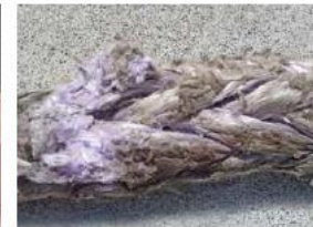
Visual inspection of yams on rope in this sample shows heavy cutting on two adjacent strands, but only moderate surface abrasion (darker areas on the surface of the strands).
