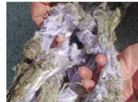
Visual inspection of interior yams shows wear from abrasion or cutting.
