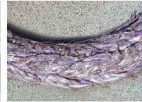
Inspect for excess surface wear on rope
