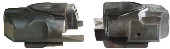
Figure WC-7: Schematic (top) and photo of Upper and lower shearing blind rams. Photo courtesy GE Oil & Gas. IADC drawing at top.
