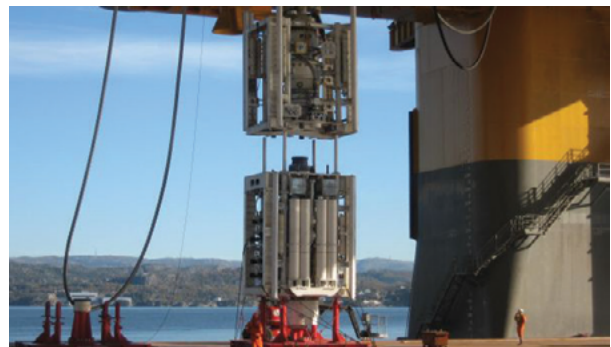
Figure WC-3: Schematic (top) and photo of typical subsea BOP stack. Photo courtesy GE Oil & Gas. IADC drawing at top.
