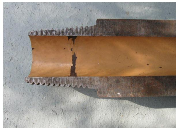
**Figure DS-6:** Plastic coating in the pin bore acts as a stress coat and serves as an early indicator of pin stretch.
