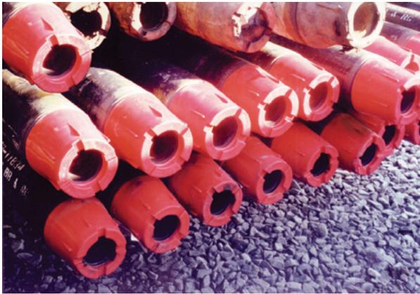
**Figure DS-7:** Thread protectors will prevent most tool-joint damage that can occur during moving or racking.
