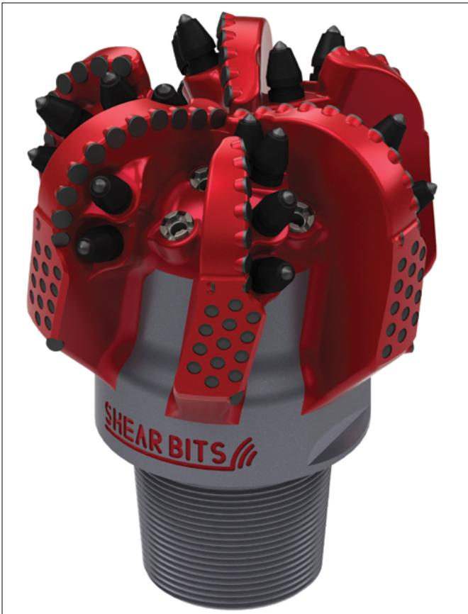
*Top:* Shear Bits' Pexus bit, a PDC and carbide hybrid bit, uses carbide elements to shear hard formation to protect PDC cutters from damage. *Bottom:* The Pexus bit has been used extensively in Western Canada to drill glacial till, comprised of a hard top layer of boulders and gravel, and a soft bottom layer of sand and shales.
