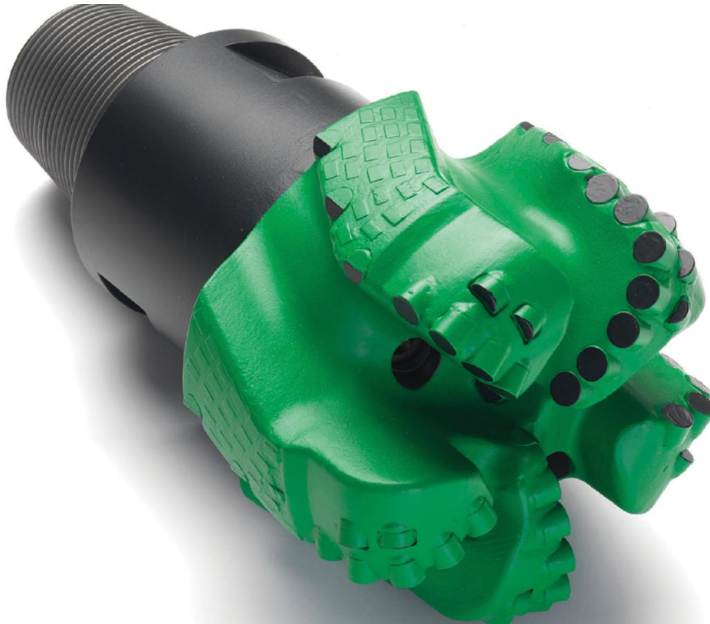
*The Tercel MicroCORE drill bit applies PDC cutters to the outer diameter of the bit and eliminates cutters in the center of the bit. This placement helps to focus energy on faster-moving outer PDC cutters. Originally designed to produce "microcores" through the center of the bit for geological evaluation, the bit was recently optimized to focus on increasing ROP. The bit has been used in places such as the Eagle Ford, Bakken, the Tunu Field in Indonesia and the Southern North Sea.*
