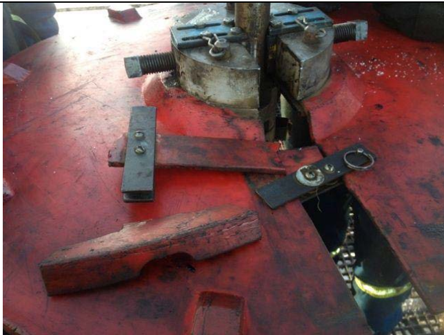
The gate piece of the rod wheel broke away, striking a worker.
