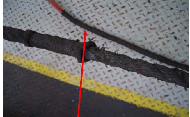
The outer sleeve of this tag line created a snagging hazard.
