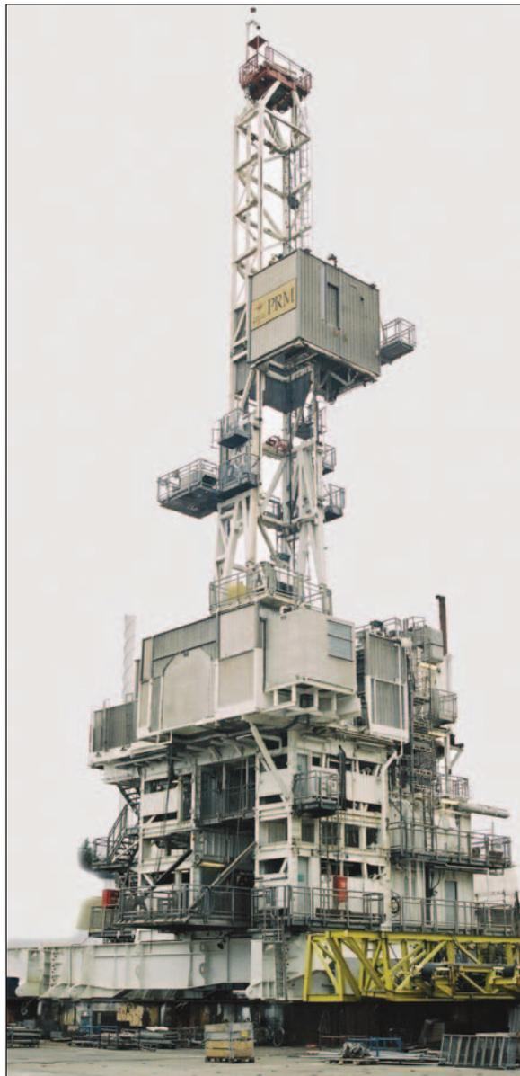
**Polaris Rig Management’s 1,000-hp modular rig was designed so that it offers flexible layout configurations and can be mobilized either as a single lift or on a piece-small basis via a series of smaller lifts.**
