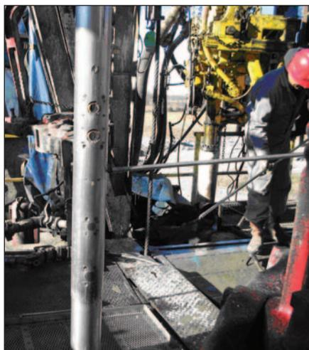
**A PathFinder Energy Services engineer on the rig floor installs a Cs137 gamma ray source into the Slim Density Neutron Standoff Caliper mandrel.**
