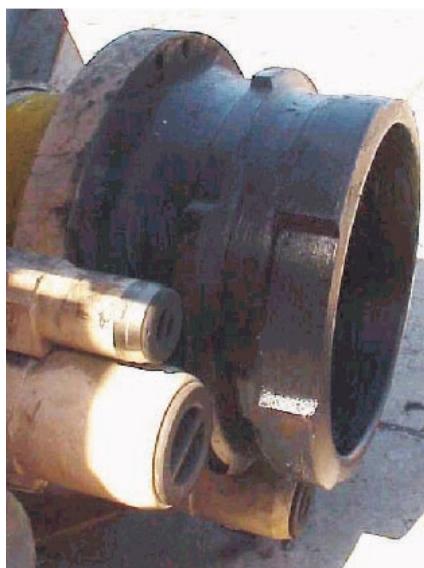
Clip connector developed by IFP (pin side is shown) offers faster, safer make-up/breakout.
