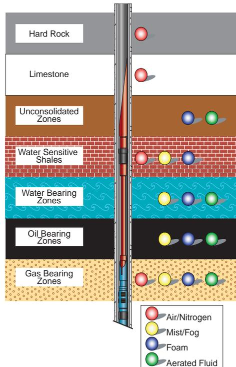
Figure 1: Operators currently use 4 types of UBD drilling fluids: air/nitrogen, mist/fog, aerated fluid and foam.
