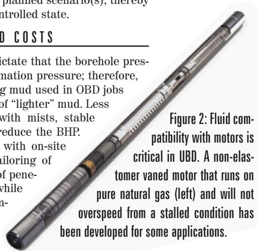
**Figure 2: Fluid compatibility with motors is critical in UBD. A non-elastomer vane motor that runs on pure natural gas (left) and will not overspeed from a stalled condition has been developed for some applications.**
