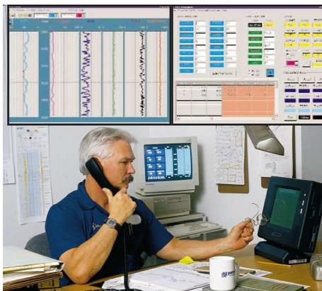
The work station: Individual remote workstations displaying data digitally and graphically enable members of the drilling team to become more focused and productive. Insets: State-of-the art displays include drilling parameters with TVD and lag correction(left inset) and real-time hydraulics (right inset).
