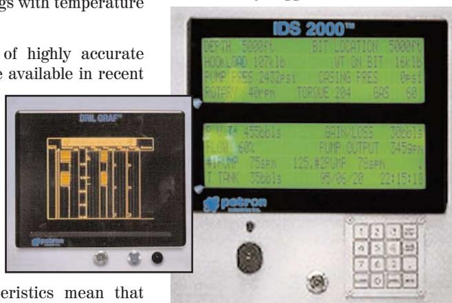
Driller's display: An alarmable alphanumeric display gives the driller tight control of key drilling parameters. Digits should be large enough to see from a distance. Inset: Optional graphical and gauge displays driven from the driller's console are useful supplements.
