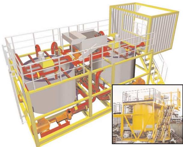
**Slurrification:** Once transported to the slurrification system via screw conveyors, cuttings are mixed with water and sometimes chemicals. Through a combination of special mix-tank screw agitator, grinding pumps, grinding mill and classification shaker, the cuttings are transformed into a pumpable slurry with a predetermined particle distribution.
