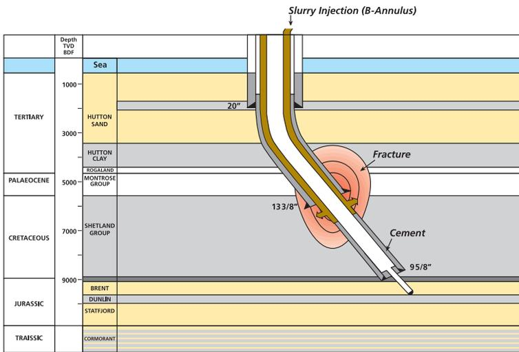
**KCA Drilling determined that reinjection was the optimum method to achieve total containment of mineral-oil contaminated cuttings. After revamping platform topsides to accommodate injection equipment, the team selected the recipient formations. More than 100 existing wells were screened to identify test candidates. Reinjection began in earnest in 1999 and has proven successful.**
