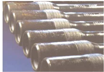
**New hardbanding compound:** Casing-wear tests found that ICO's new hardbanding compound significantly outperformed uncoated steel tool joints and those hardbanded with spherical tungsten carbide. The tests determined a wear factor for the ICO material nearly one-fourth that of the next-best performer.
