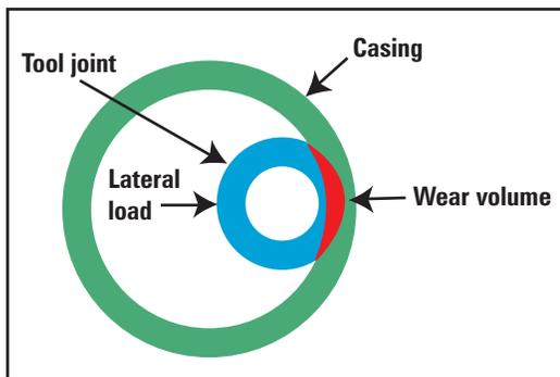
**Casing wear culprits:** Casing wear occurs when drillstring tension holds the rotating tool joints against the casing, explains Maurer Engineering (left). As shown in the inset above, this contact wears a crescent-shape groove in the casing. The outside of the tool joint also wears.
