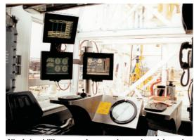
All of the drilling operations can be monitored from the driller's cabin of Helmerich & Payne's Flex 3 rigs. These rigs also feature AC drive motors and an integrated top drive drilling system.
