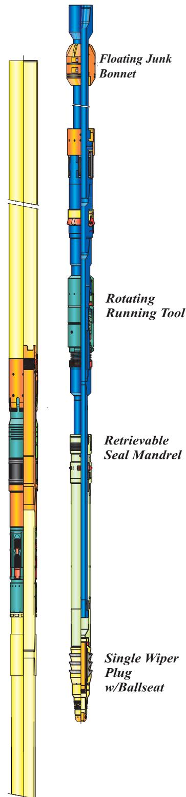
**Retrievable packer:** While retrievable cementing packers are not new, a recent new twist is use of a retrievable-seal mandrel as an upper cementing pack-off, with the lower isolating pack-off sealing the inside of the liner. No drillable pack-off below was necessary.
