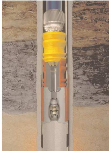
**Subsea release cementing plugs: A new approach to liner cementing is a subsea plug comprised mainly of polyurethane. Since it contains little aluminum, less of that element must be drilled. This has reduced drill-through times to less than 2 hours in several GOM wells.**
