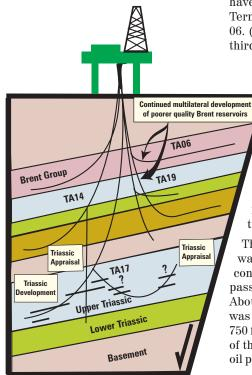
4 TAML Level 4 multilaterals were successfully installed in Shell Expro's Tern Field by early '99—TA-14, TA-19, TA-17, and TA-06. The 5th multilateral, TA-16, then had only 1 lateral.
