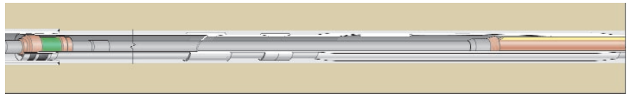
Multilateral junction construction begins with installation of a pre-milled casing window.
