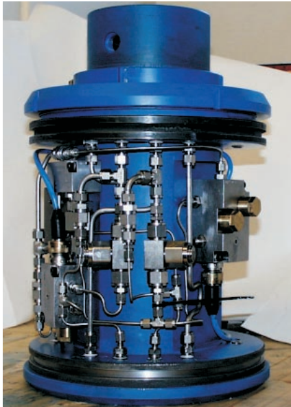
Figure 2: Electro-hydraulic control pod for DST operations has undergone extensive testing.
