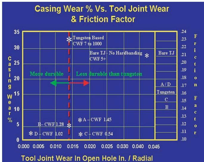
One, though, has a drastically lower casing wear factor of 0.54, with the others grouped in a narrow range of 1.02 to 1.45.
