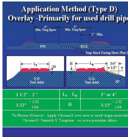
Apply a  $3/32$ -in. thickness (+/-  $1/32$  in.) by 3-in. long raised hardbanding on the tool joint box OD. Start the hardbanding  $1/4$  in. from the taper to allow elevator clearance. Apply a  $3/32$ -in. thickness (+/-  $1/32$  in.) by  $1\frac{1}{2}$ -in. to 2-in. long raised application to the tool joint pin.
