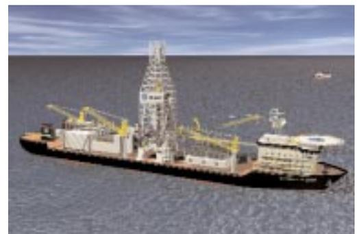
SPE/IADC 52858: Global Marine's 5th-generation 456 class features a unique arrangement and type of thrusters to slash weather-related downtime. The rig also employs horizontal/vertical pipe handling.
