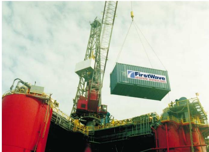
During offsite services, all tools and equipment needed for the job are brought to the site. In the case cited in this article, the gear included a 20-ft fully equipped con-ex box containing the tools and an 8-bank welding machine.
