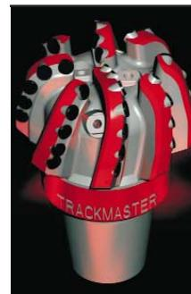
IADC/SPE 59185: PCD cutters were modified and applied to a casing-sidetracking mill. The mill could cut a window in casing and drill a rat hole in formations with compressive strengths up to 40,000 psi.
