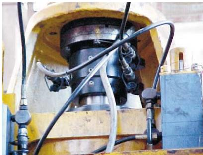
**IADC/SPE 59107:** A new hydrodynamic washpipe assembly has demonstrated significant economic advantages. This sealing system has cut drilling costs for the Woodside Goodwyn A platform by some US \$500,000 on one well.
