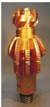
IADC/SPE 59239: New bi-center bits can drill out and then continue to drill ahead. ROP, directional control, and hole quality have improved. 3 field tests in the deepwater Gulf of Mexico have saved \$560,000 in trip costs.
