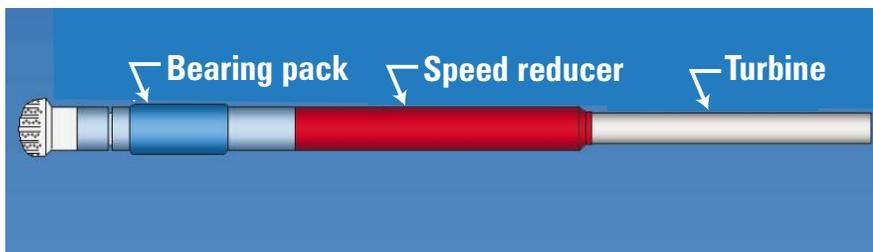
IADC/SPE 59156: A new, advanced geothermal turbodrill uses a gear box to increase the torque 13-fold and reduce the speed of the turbodrill to 80-120 rpm, suitable for rollercone or PDC bits.
