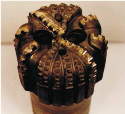
**IADC/SPE 59154: A new high-power slim-hole drilling system, capable of drilling twice as fast as conventional systems, consists of a double length PDM motor and a hybrid PDC/TSP bit.**
