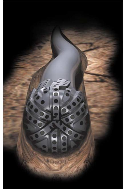
**IADC/SPE 59113:** A new PDC bit was run successfully in the Huamampampa formation in Tarija, Bolivia. In a long, 8 1/2-in. hole section with 10%-90% shale, the bit type drilled to TD with a higher overall ROP than any offset.
