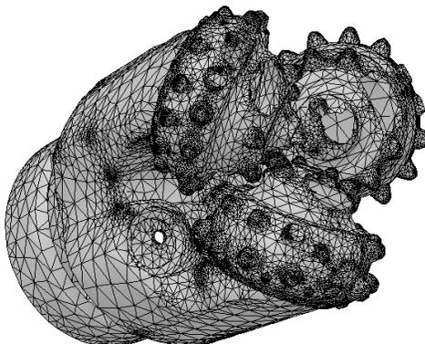
IADC/SPE 59111: 3-d computational fluid dynamics (CFD) models of the entire flow field between rollercone bits and boreholes have been used to identify fluid dynamic parameters that are characteristic of bits that drill well in bit and bottom balling environments. From this, a nozzle system has been developed with characteristics of both bit and bottom balling nozzle systems.
