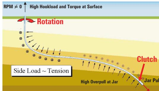
IADC/SPE 59234: The down-hole clutch is designed to enhance jarring effectiveness, especially in horizontal and other high-drag wells. The tool is placed above the jar.
