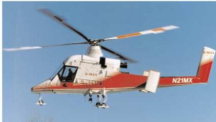
Kaman's heavy-lift helicopter K-MAX features 2 separate forward rotors, which eliminates the need for a tail rotor. The 'aerial truck' showed its stuff at the '99 OTC, making flights around the Houston Astrodomain parking lot while carrying as much as 5,500 lb of equipment.
