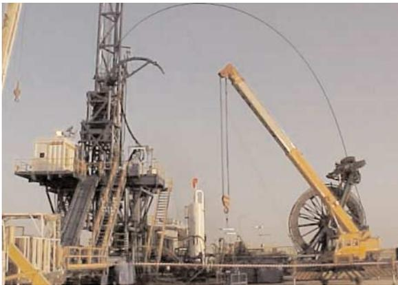
8-plus years of horizontal drilling; Baker Hughes began drilling horizontal wells in Oman in 1990. Well designs have since evolved, as has the equipment. In February 1999, Baker Hughes brought the first coiled tubing drilling rig to Oman. The fully automated Galileo 3 is able to deploy drilling and work coil strings as well as handle pipe via a conventional mast.
