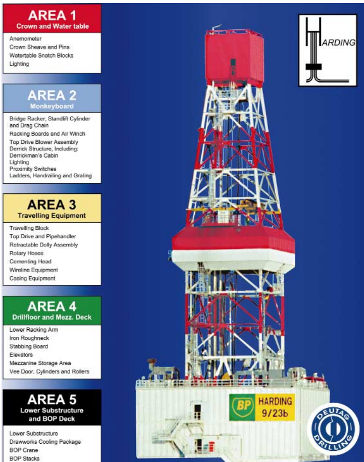
Figure 1: The Harding drilling team identified 336 potential “dropped objects” in the derrick and substructure as part of a comprehensive effort to eliminate the problem. The next step was to identify all derrick and sub-structure operations. Finally, the team sub-divided the derrick and sub-structure into 5 manageable derrick inspection areas. Colour codes were used to ensure check sheets were referenced to the appropriate area.
