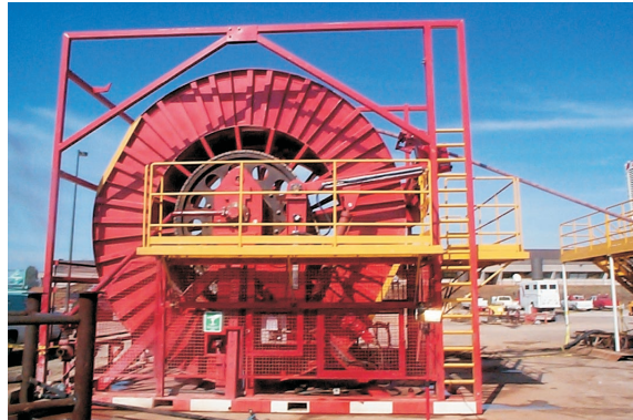
Continuous coil of carbon fiber laminate drill string is a feature of Halliburton's new Anaconda well construction system.
