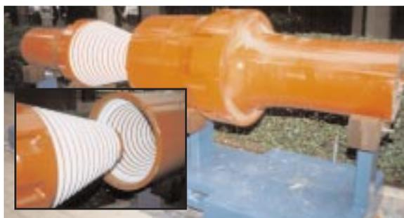
Together, the 579 joints measured 17,370 ft and weighed 4,700 short tons. The pipe wall is some 4 3/4 in. thick through the body, with ODs of 28 in. at the joint and 15 1/2 in. through the body. The pipe was a one-piece forging with a trepanned bore. ■
