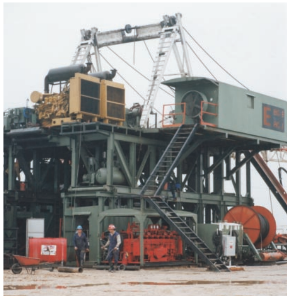
The new diesel engines on Big E Drilling Co's Rig No 1 provide 210 additional horsepower while burning 10-20% less fuel.
