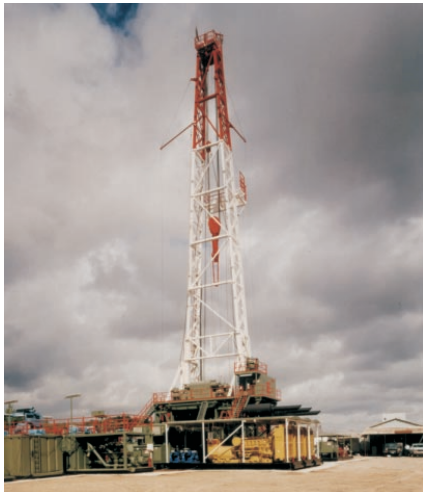
Big E's Rig No 5 is a 1,500-hp SCR unit with a 20,000-ft depth rating and new engines.
