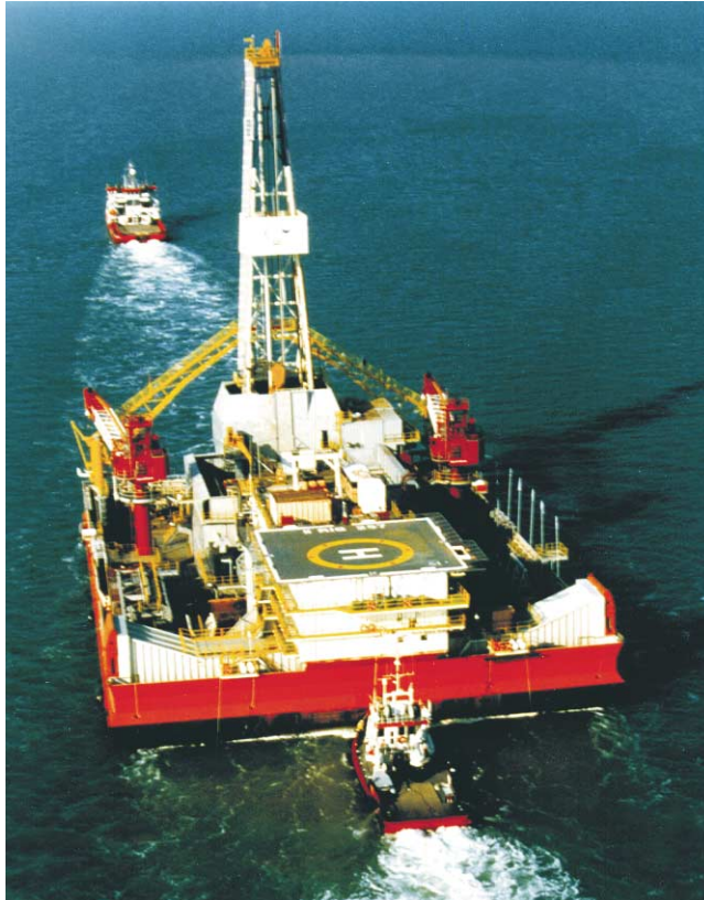
Parker Rig 257: Designed for Caspian Sea operations, Parker Rig 257 was upgraded to operate as an arctic drill barge. The rig was designed to meet 4 criteria: environmental and personnel safety; remote, shallow-water operations; severe, arctic weather; and an HPHT, H 2 S reservoir.
