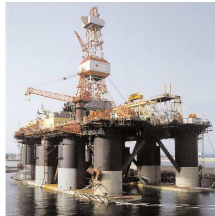
Newly launched: Saipem's Scarabeo 7 was recently christened. The converted semi is capable of drilling in water depths to 1,500 m.
