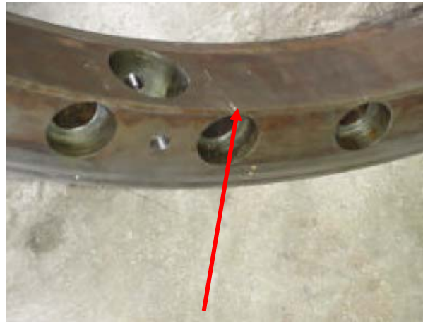
Cracked Wall in Ring:
